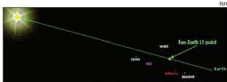
Diagram from Isro's earlier situational analysis showing orbital positions of various operational spacecraft at Sun-Earth L1 point with the expected location of Aditya-L1
